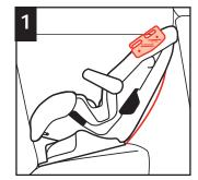
Rear Facing Use: 5-35 Connect and tighten harness straps prior to installing in vehicle. Place child restraint rearfacing in the back seat. lbs. With child restraint in the most reclined position, (2.3-16 kg), 19-36" (48-91 cm) make sure level lines on shoulder belt positioning quide are level with ground. Adjust child restraint if needed. **NOTE:** Tuck top
